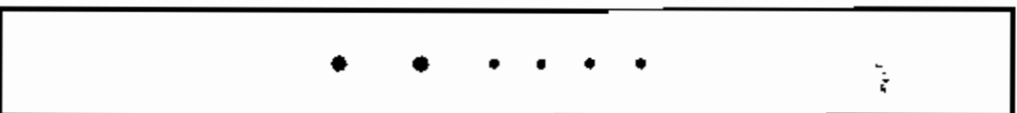
EXAMPLE 5: TWO 1/16" (1.6 mm), FOUR 1/32" (0.8 mm) DISCONTINUITIES
