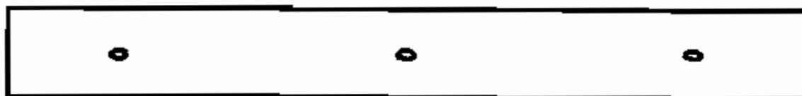
EXAMPLE 3: THREE \frac{1}{8} " (3.2 mm) DISCONTINUITIES
