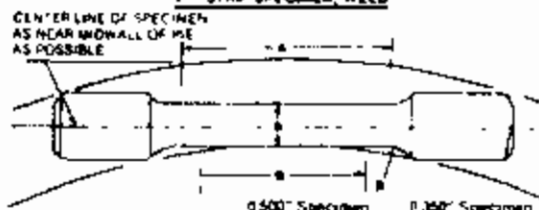
F - STRIP SPECIMEN, WELD
